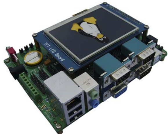
Embest SBC9261-I Single Board Computer
